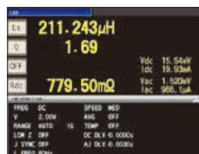
L, Q and Rdc continuous measurement screen L and Q (1 kHz, 1 mA constant current measurement) and Rdc (DC measurement) display screen
