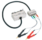
FOUR-TERMINAL PROBE L2000 Cable length 1 m (3.28 ft), DC to 8 MHz, impedance characteristics of 50 Ω, 4-terminal pair configuration, measurable conductor diameter: ø0.3 mm (0.01 in) to 5 mm (0.20 in)
