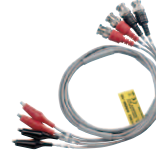
FOUR-TERMINAL PROBE 9500-10 Cable length 1 m (3.28 ft), DC to 200 kHz, impedance characteristics of 50 Ω, 4-terminal pair configuration, measurable conductor diameter: ø0.3 mm (0.01 in) to 2 mm (0.08 in)
