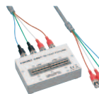
FOUR-TERMINAL PROBE 9140-10 Cable length 1 m (3.28 ft), DC to 200 kHz, impedance characteristics of 50 Ω, 4-terminal pair configuration, measurable conductor diameter: ø0.3 mm (0.01 in) to 5 mm (0.20 in)
