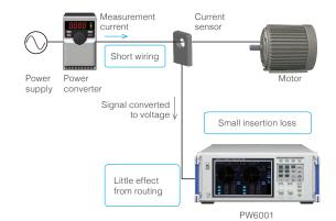
Compared to the direct wire connection method, measurement with conditions closer to the actual operation environment of a power converter is achieved.
