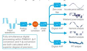
\* AAF (Anti-aliasing filter): This filter prevents aliasing errors during sampling.
