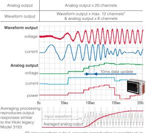
\*During waveform output, accurate reproduction is possible at an output of 1 MS/s and with a sine wave up to 50 kHz.
