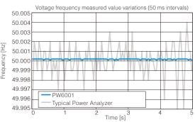
\* ±0.01 Hz fundamental accuracy is defined for cases where the data update is over 50 ms. Please contact us for even more precise frequency
