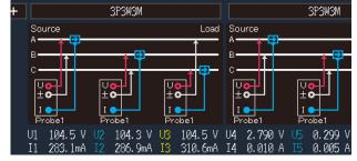
Wiring confirmation function, to avoid wiring mistakes
