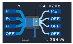
Setting up efficiency calculation formulas for power conditioners and similar equipment is simple on the dedicated screen. Simultaneously display loss and efficiency calculations for a maximum of four systems.
