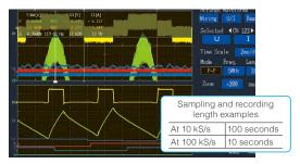
In addition to level triggers, Ver. 3.00 now includes event trigger functions triggered by RMS value and frequency fluctuations. Cursor measurement and waveform zoom functions also render oscilloscopes unnecessary for waveform analysis.
