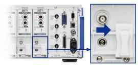
Wideband probe terminal: Slide the cover to the right. When connecting 3273-50, 3274, 3275, 3276, CT6700 or CT6701
