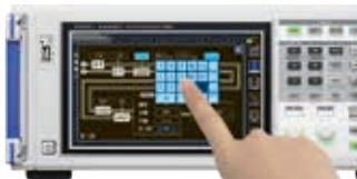
Enter current sensor phase characteristic representative value as phase compensation value
